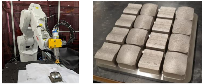
Fig. 2. a. Hardware setup b. Printed wavy and dome component
