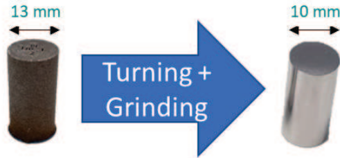
Figure 1. Specimen for X-ray and Archimedes density measurement
